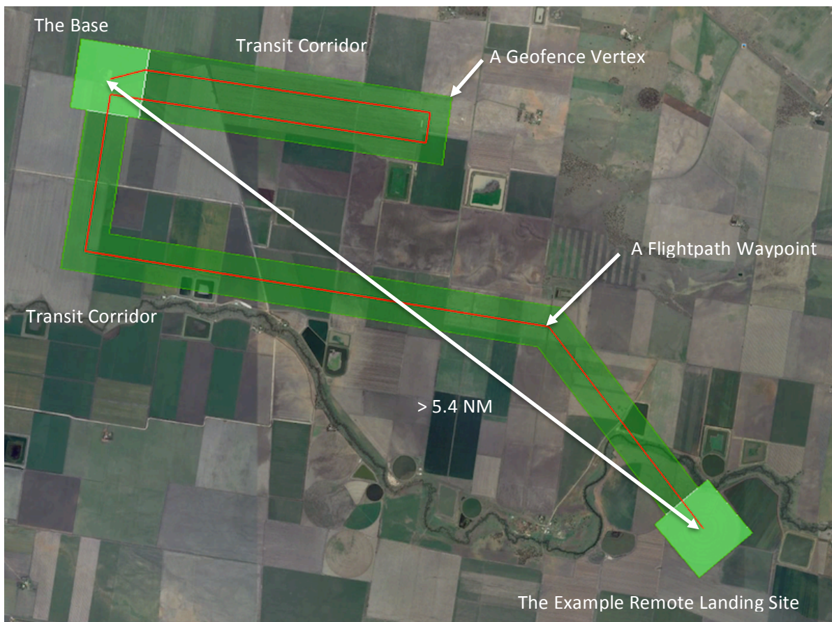
Figure 1: An example layout for the Geofence areas of the Medical Express competition. Note that this figure is an example and does NOT show the actual Transit Corridor or Remote Landing Site.
