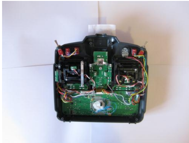
6 - RC Transmitter with back cover removed
